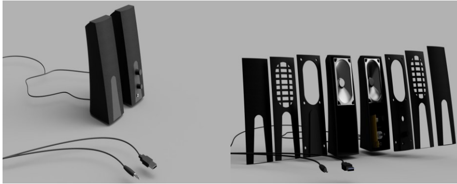
Figure 9: Photorealistic renders of the designed speakers (left) assembled components (right) exploded assembly (Student provision)
